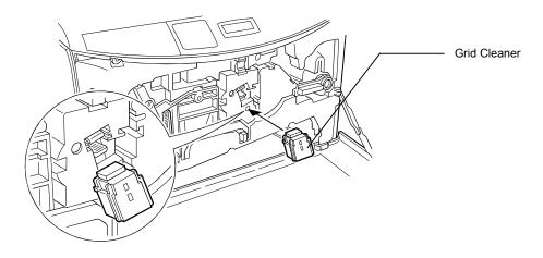
3. After attaching the grid cleaner, slightly lift the main charger unit and repeat the action of slowly pulling the cleaning knob in and out at least five times. This will clean the grid inside the main charger unit.
